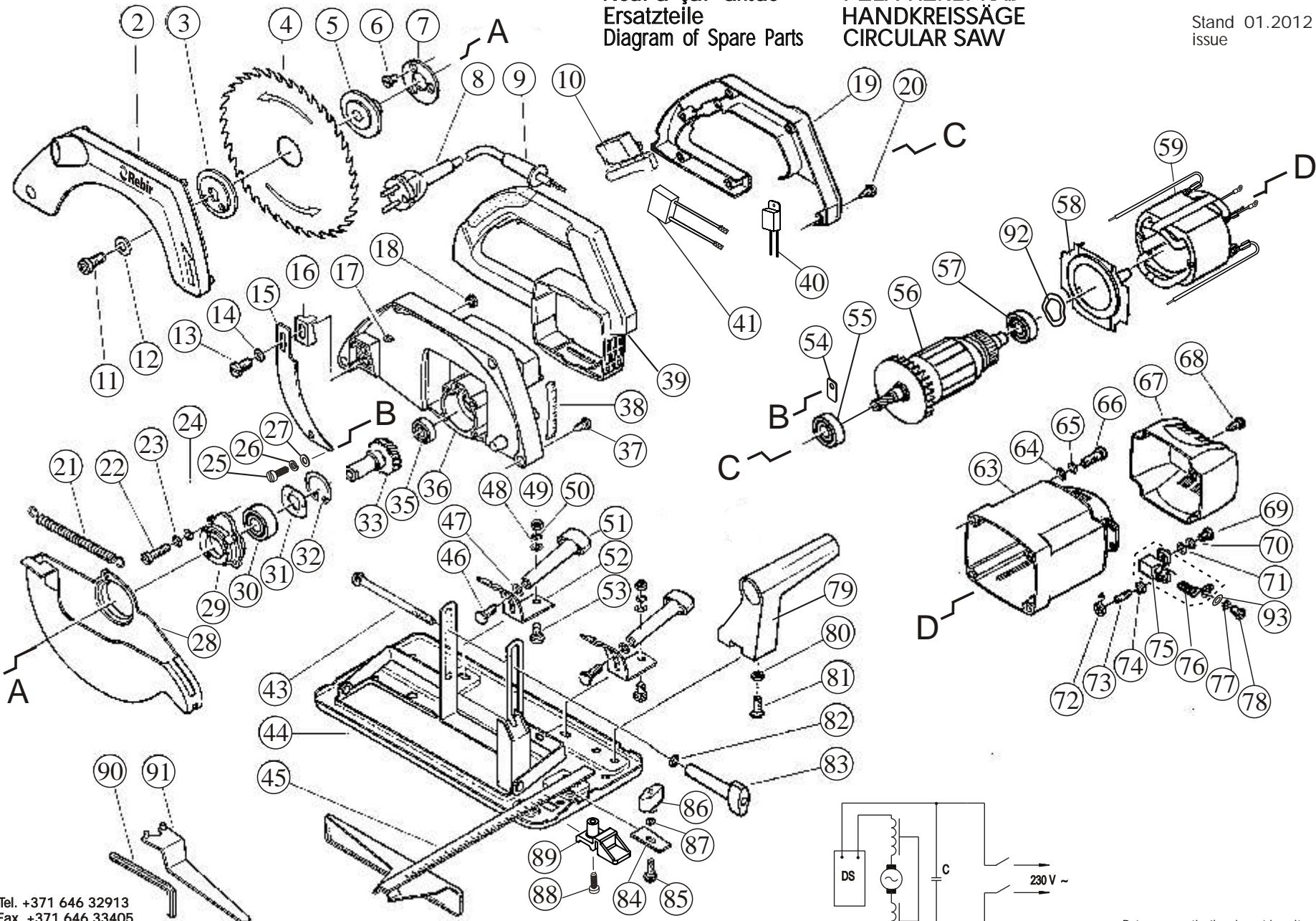
Spare parts supply via REBIR service offices. When ordering spare parts quote power tool type and date of manufacture indicated per machine label, date as per Diagram of Spare Parts, desired spare part number and name as per List of Spare Parts and desired quantity.
