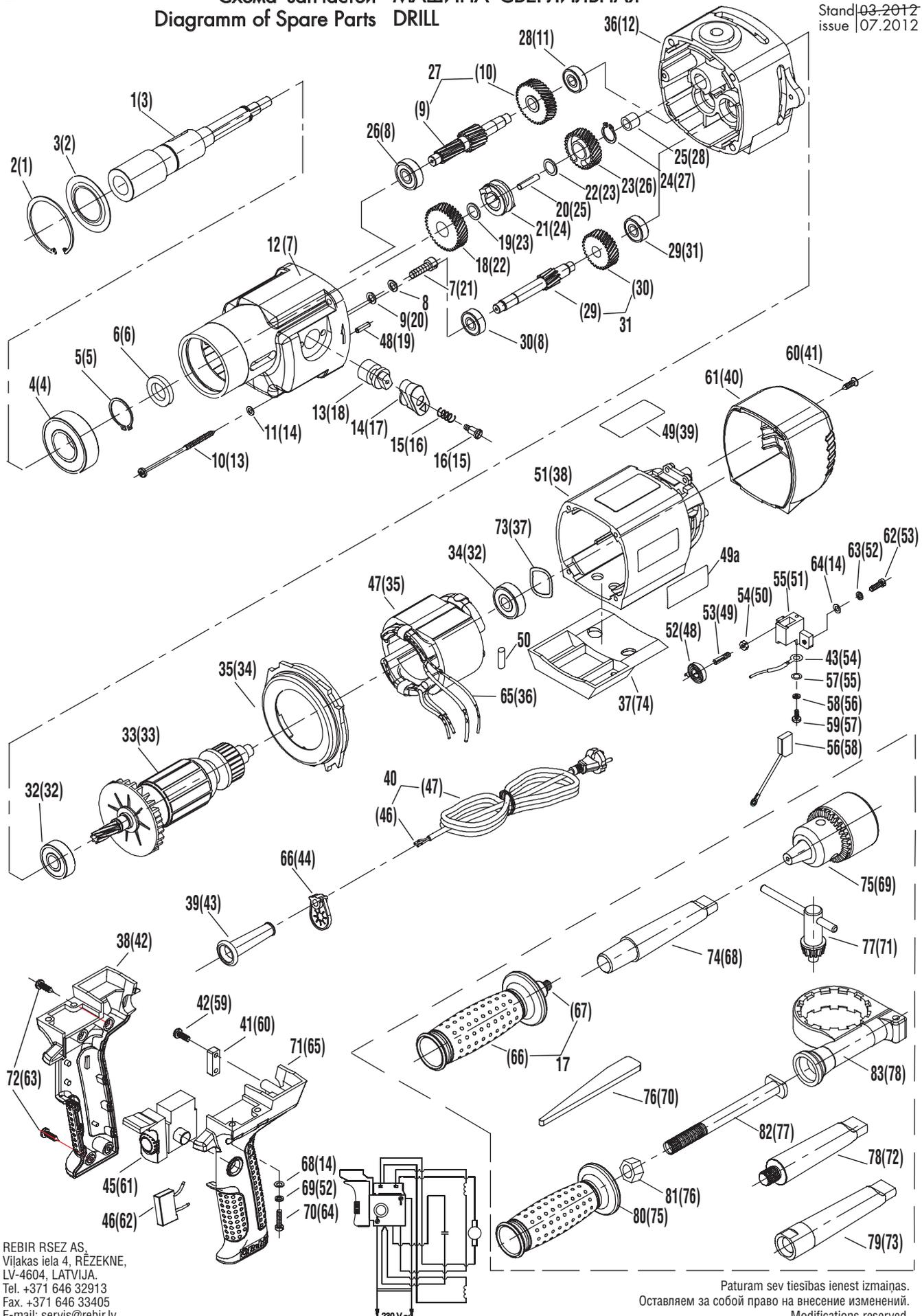
Spare parts supply via REBIR service offices. When ordering spare parts, please quote power, tool type as and date of manufacturing indicated per machine label, date as per Diagram of Spare Parts, desired spare part number and name as per List of Spare Parts and desired quantity.
